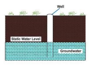
Figure 5-1 — Static water level.
