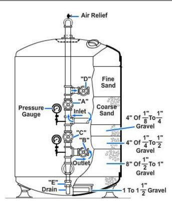
Figure 5-16 — Pressure-type water filter.
