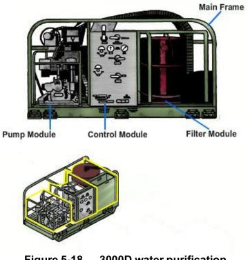
Figure 5-18 — 3000D water purification system.
