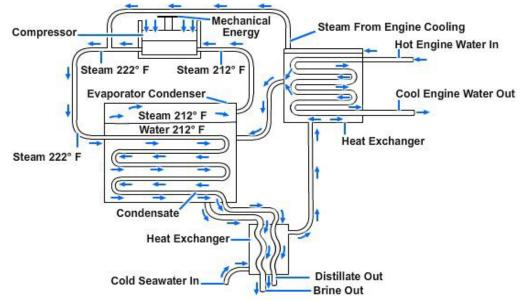
Figure 5-11 — Flow diagram-thermocompression distillation.
